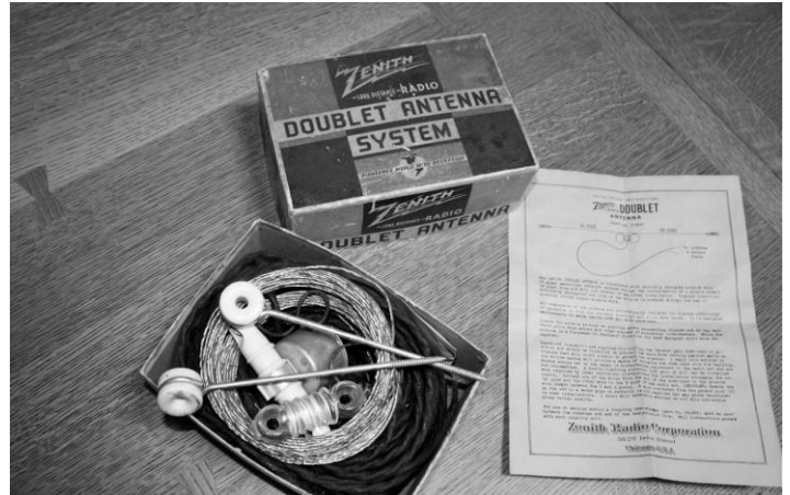
A 1930s era Zenith Doublet (or dipole) Antenna System. The antenna wire feed to the plug connects to the cap in the center of the box. The two coils of wire would then be on the unwound from the cap and kept taut with the screws with porcelain insulators to form the dipole antenna. Courtesy of David Wilson.
